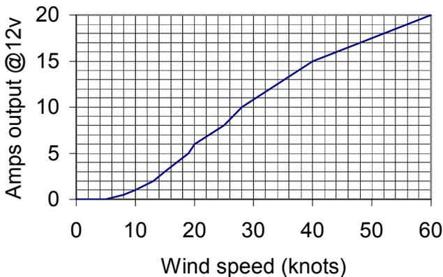
Note: Amps output of a 24v model will be half shown above.
