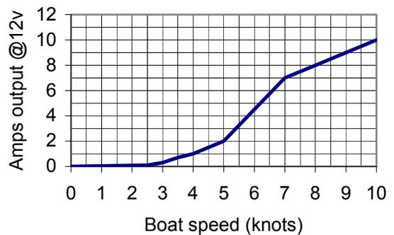
Note: Amps output of a 24v model will be half shown above.
